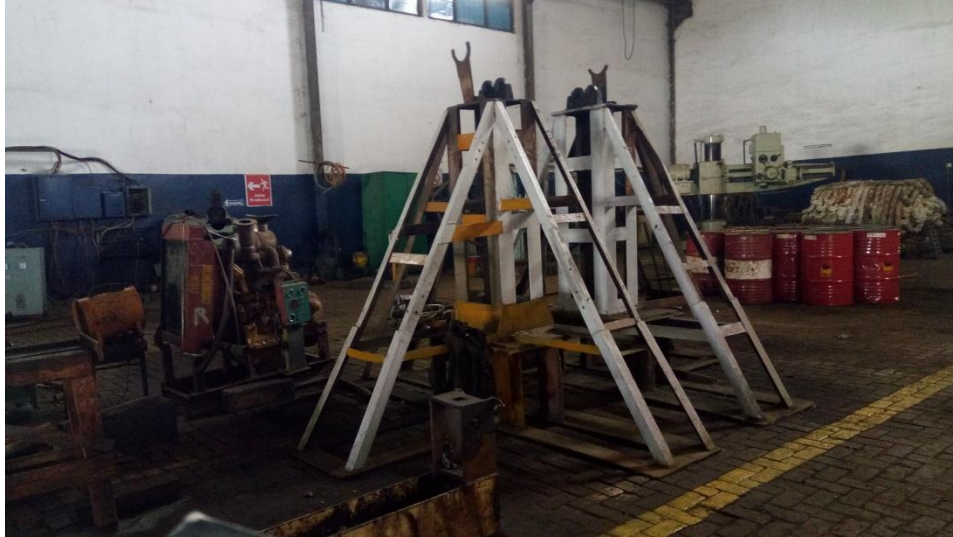
Gambar 4 : Alat balancing propeller PT.Rukindo
