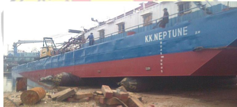
**Gambar 1 Dock Sistem Airbags (Dok Sistem Balon)**
