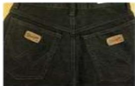
**H. Poor shape of leather patch due to overheating**
