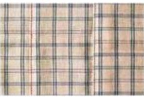
A close-up photograph of a fabric seam with a plaid pattern. The two pieces of fabric being joined do not have matching plaid patterns, resulting in a mismatched appearance at the seam.                  |
