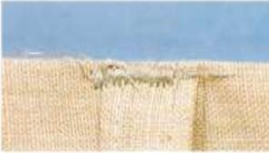
A close-up photograph of a light-colored fabric seam. A bar-tack, which is a reinforcement stitch, is placed at an angle that does not align with the fold of the fabric, illustrating incorrect placement. |
