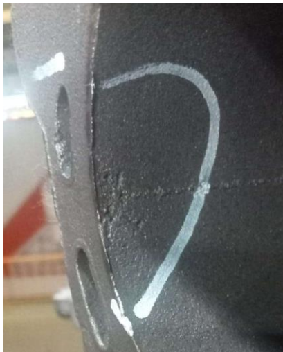
Gambar 1.5 Defect jenis sand inclusion/inklusi pasir
