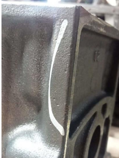
Gambar 1.4 Defect jenis Gas hole/porosity
