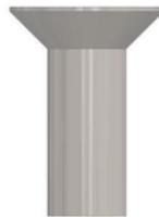
Gambar 2. 5 Solid Rivet Countersunk
