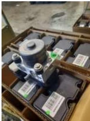
**Gambar 1.3** Modul ABS (*Anti-Lock Braking System*)
