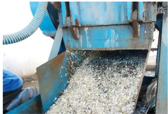
Our custom flaking machine prepares recovered ocean plastic for recycling by washing it and shredding it into small flakes. This machine can process up to 3 tons of plastic every eight hours depending on the type of plastic.
