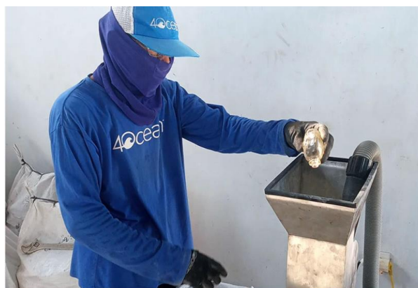
The glass crusher pulverizes our recovered ocean glass to prep it for recycling. Once crushed, recovered ocean glass is transported to recycling partners who use it to make new products like our clear glass bracelet beads.
