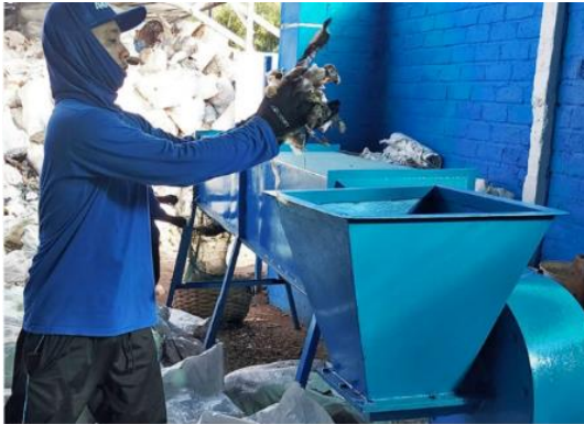
The river trash we collect is often covered in dirt and mud. The trash shaker is used to remove contaminants from recovered debris before it's sorted.
