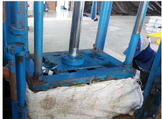
Our custom baler compresses sorted plastics into a bale that's easier to transport and can process up to 10 tons of plastic every eight hours, depending on the type of plastic.
